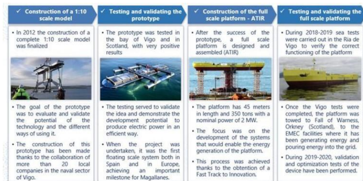
Figure 1. Evolution of the Magallanes Tidal Energy Technology
