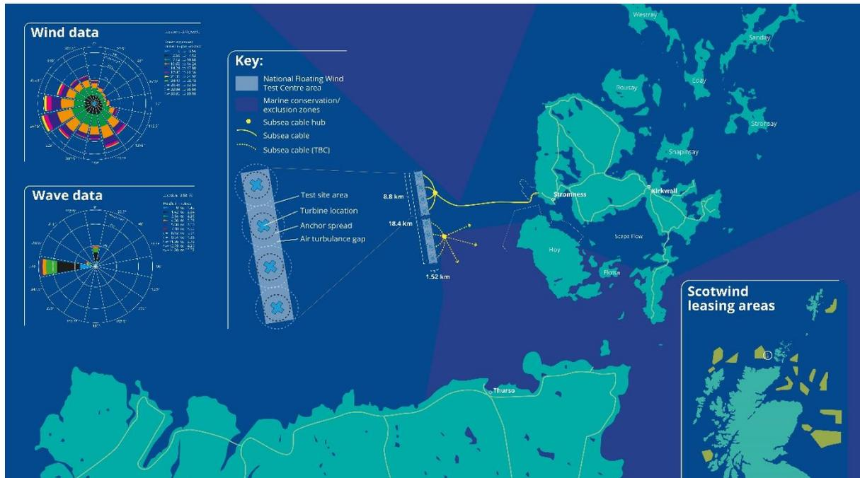
Figure 6 | Proposed floating wind test centre location and wind and wave roses
