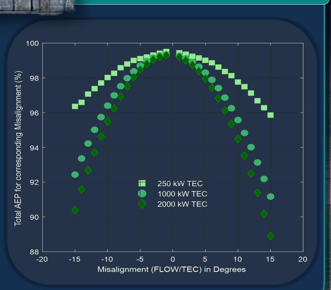
Active yaw systems can aid TEC concepts when they operate beneath the rated velocity to ensure maximum energy is captured – above the rated capacity the TEC can still operate at maximum efficiency due to the surplus in velocity magnitude.
