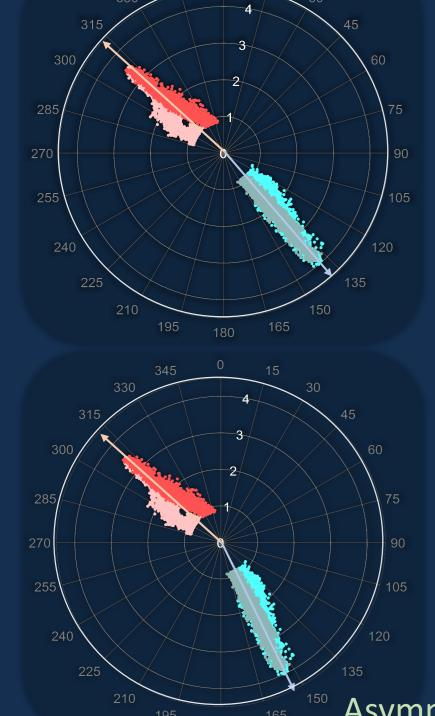
Tidal test sites suffer from both current magnitude and current direction variations. Tidal energy converter (TEC) developers deploy their device under the influence of a site characterisation carried out by Acoustic Doppler Current Profilers (ADPCs) [1]. These instruments provide current velocity and directionality data to inform developers on turbine placement and orientation.
