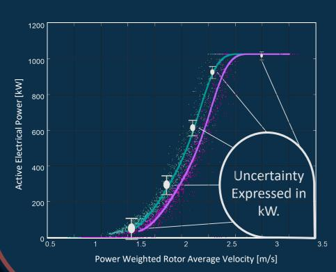
The purpose of the assessment of power is the production of the power curve, this requires a robust flow velocity measurement to be paired with the corresponding electrical power of the device.
