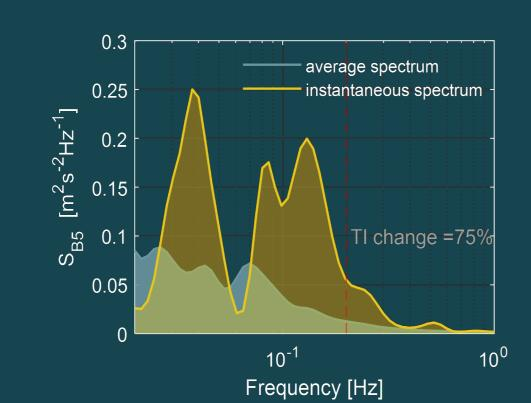
Wavelets allow detection of transient, energetic turbulent bursts. At the FoW test site, these can occur at frequencies which are significant tidal turbine loading, and can result in turbulence intensity increase up to 80%.
