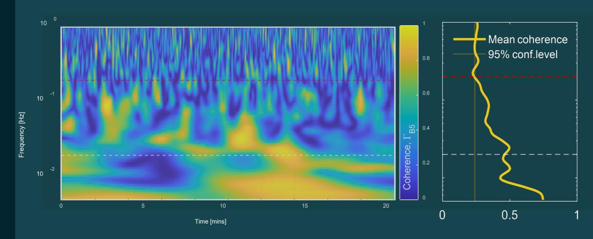
Coherency, which can only be analysed with average on Fourier methods, can be detected at each time instant with wavelets. This allows to detect the passing turbulent large eddies in the flow.
