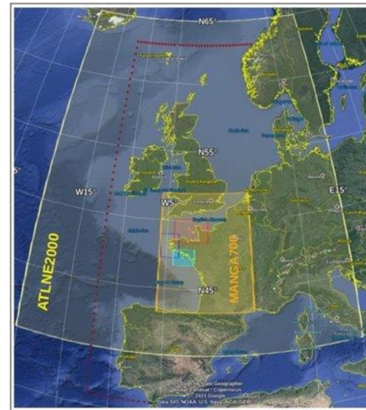
IFREMER tidal atlas domains with resolutions about 250m (coastal), 700m (France) and 2km (NE Atlantique) Red dots represent the domain open boundaries
