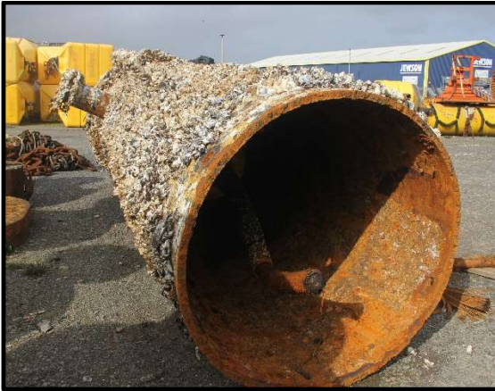
Figure 5 - The vertical subunit of the tripod surveyed on 15 September 2019. Note the thick encrustation of barnacles and mussels
