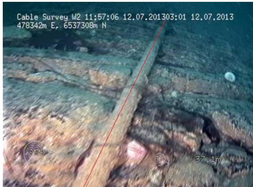
Figure 15: Wire-like material around cable W2
