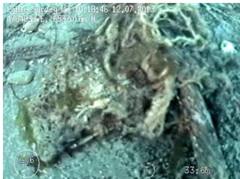
Figure 16: Wrecked fishing creel interacting with cable W3
